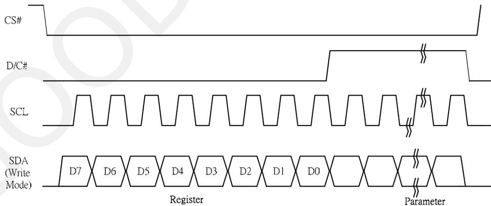
**Figure 3.5-2: Write procedure in 4-wire SPI mode**
