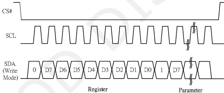
**Figure 3.5-3: Write procedure in 3-wire SPI mode**
