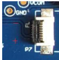
Figure 5 : Connection between DESPI-C03 and front light panel
