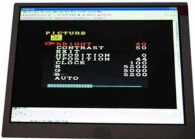
**BRIGHT:** When you press the **<Menu>** button move the cursor to the BRIGHT bar on the OSD menu, you can press **<Down>** button or **<Up>** button to adjust the image brightness value. The default value is 50, adjusting range is 0~100.
